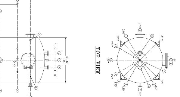
5. G.B. = GRAB BAR D.S. = DRIP SHIELD V.B. = VORTEX BREAKER N.S. = NEAR SIDE N.P. = NAME PLATE T.B. = TEE BAFFLE E.S. = FAR SIDE & = CENTER LINE
